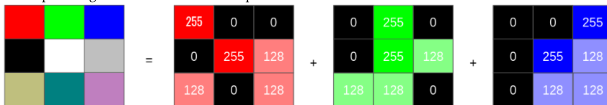
Fig. 2. Decomposition of an RGB Image into Red, Green, and Blue channels
