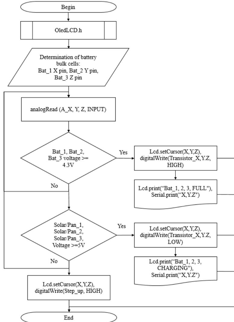
Fig. 2. The algorithm of power harvesting, power, supply and controller.
