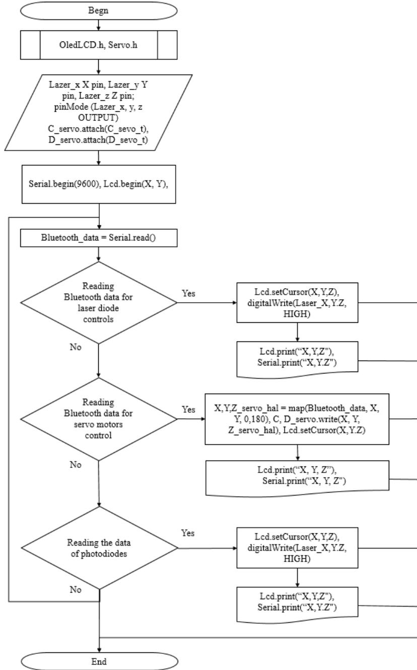
**Fig. 1.** The algorithm of laser beam control and transponder payload subsystem.
