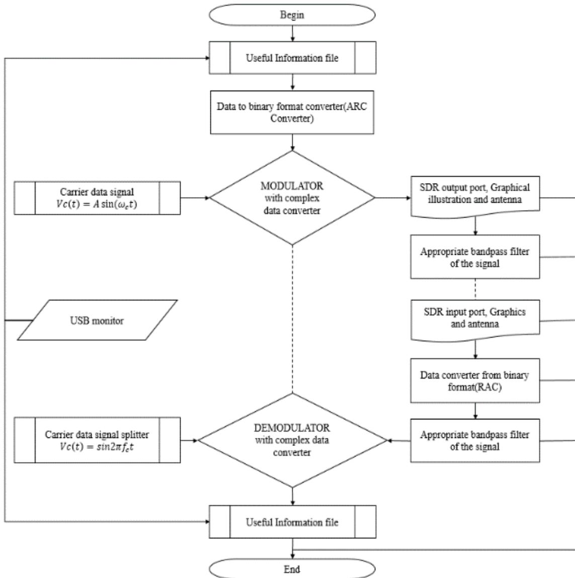
Fig. 4. The algorithm of data exchange, control, and active transponder
